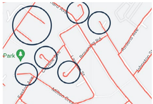
Figure 7: Illustrative map of suburban gas pipelines (red) with terminal branches circled (adapted from Solstice Energy 2024)
