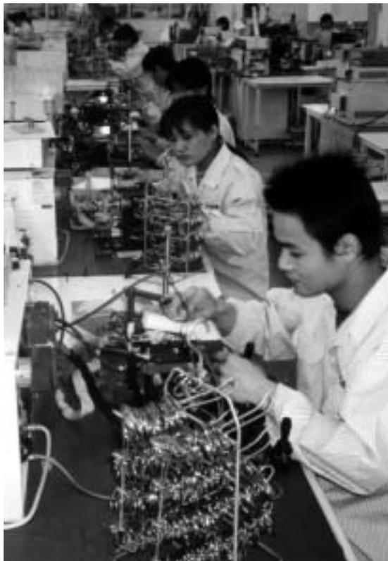
Workers soldering metal optical frames in China.
